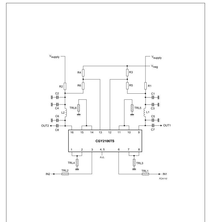
The demonstration board has been optimized for a centre frequency of 0.9 GHz. The MMIC s-parameters (typical values) are available in a range from 0.1 to 6 GHz on request.
