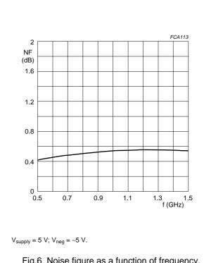
Fig.6 Noise figure as a function of frequency.
